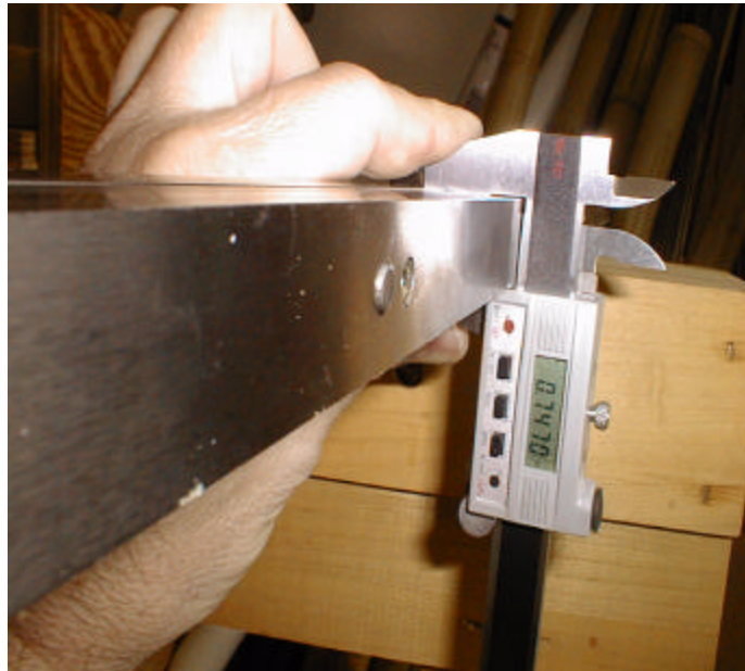
FIGURE 1. Measure Form Thickness.
