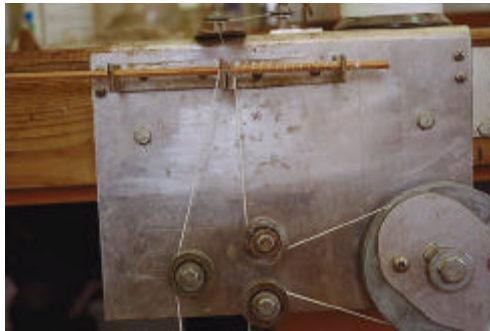
FIGURE 5. Guide Wheels and the Drive Wheel.
