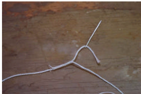
FIGURE 8. Feeding one end of the belt through the other.
